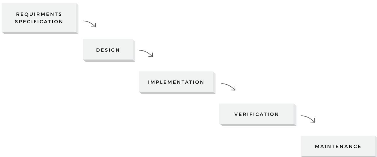
Waterfall model has a strong emphasis on planning and specifications development, which takes up to **40% of the project time and budget**. Another basic principle of this approach is the strict order of the project phases. A new project stage does not begin until the previous one is finished.
